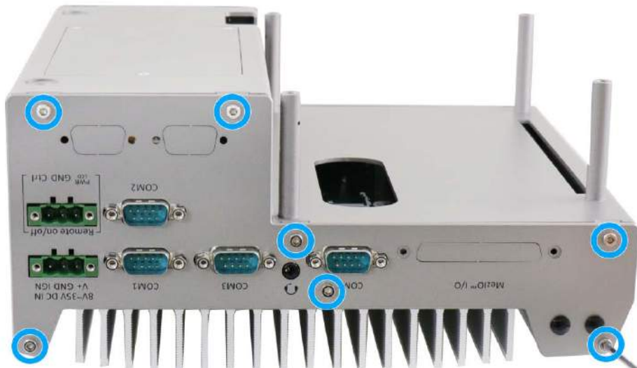
Install rear panel and secure screws
