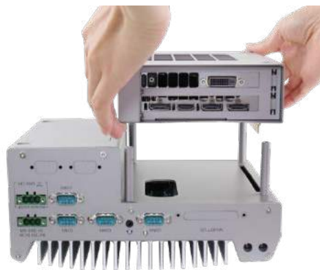
Lower Cassette module onto system
