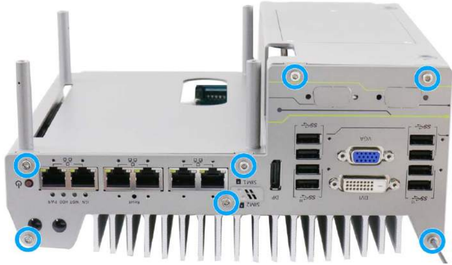
Install front panel and secure screws
