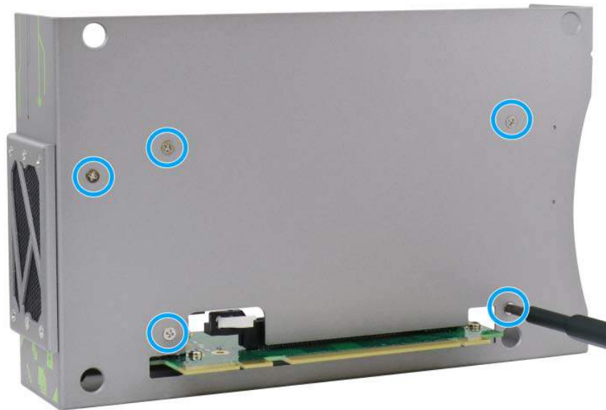
Remove air duct and bracket screws
