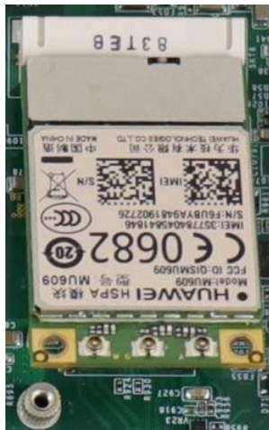
Insert on 45 degree angle
