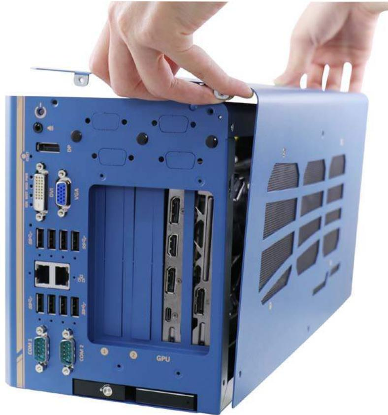
6. Once the L-shaped side panel has been removed, proceed to remove the graphics card's stabilizer plate by removing the three screws.
