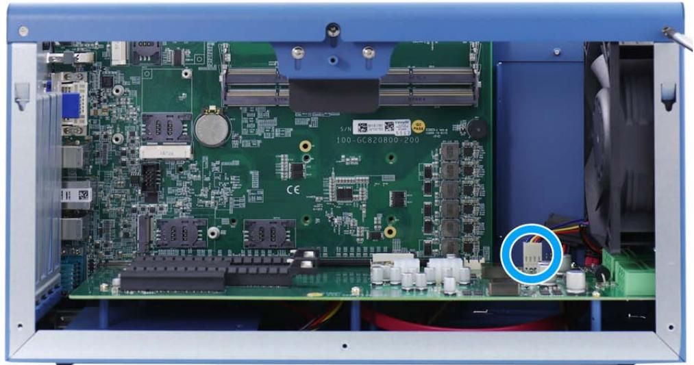
Remove 4-pin fan connector
