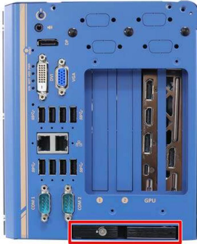
1. You may insert and install the HDD/ SSD without disassembling the enclosure. Simply lift to spring open the lever to gain access to the hot-swap slot.
