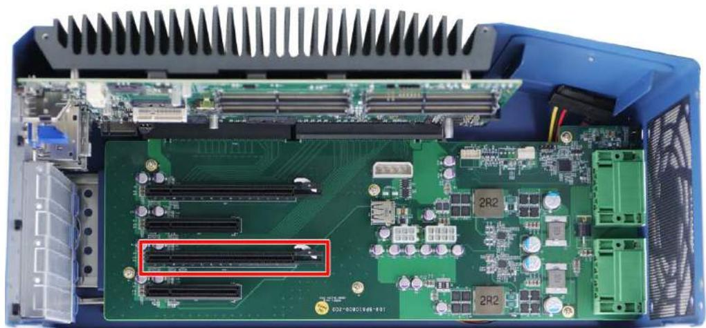
3. Remove the corresponding enclosure bezel(s) to the PCIe slot you wish to install to.
