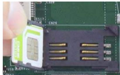
**Insert Mini-SIM card with pins facing up**
