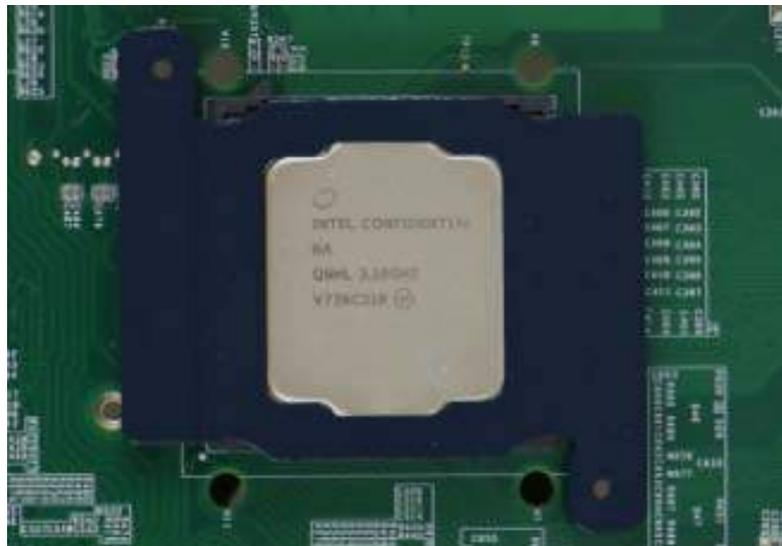
6. Turn the motherboard around and secure the bracket by tightening two M3 P-head screws.
