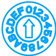
The ignition power control switch features multiple modes for pre and post ignition settings. Please refer to the section Ignition Power Control for details. Please use a flathead screwdriver to adjust the position of the ignition power control switch.
