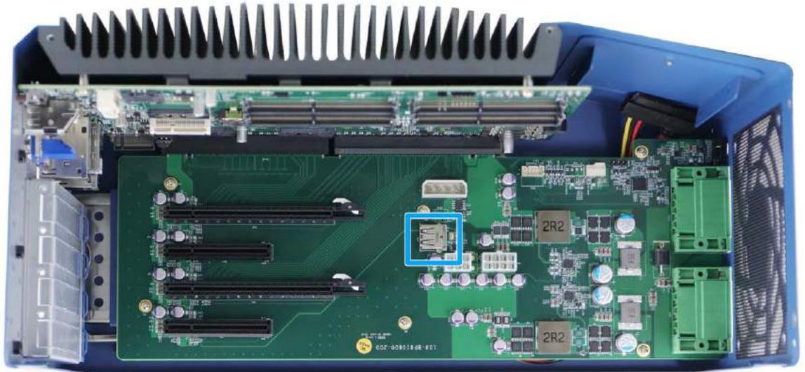
The system's extension board has an internal USB2.0 port on the PCBA. You can utilize this USB port to connect a USB protection dongle inside the chassis of the system.
