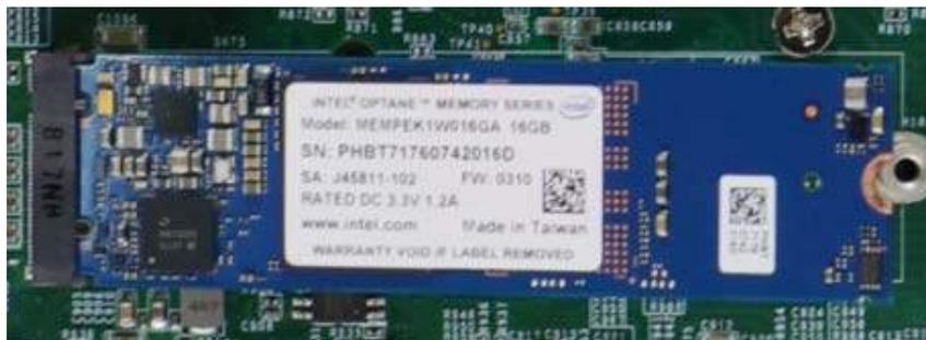
3. Gently press down and secure the module with an M2.5 P-head screw.
