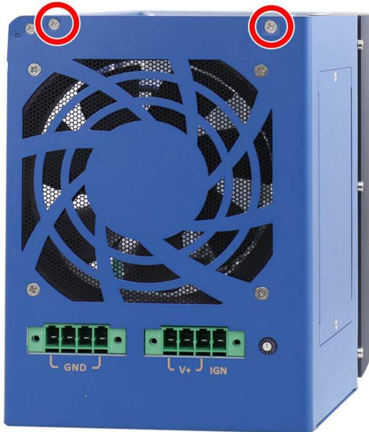
5. Lift the L-shaped side panel to separate it from the enclosure.
