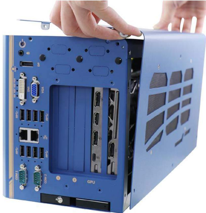
Place L-shape side panel onto the enclosure
