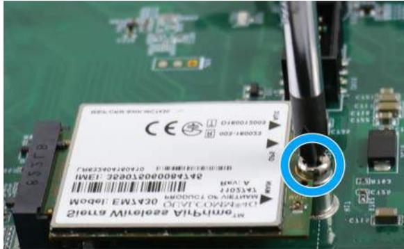
5. Clip on the IPEZ-to-SMA cable to the module and secure the antenna to the front or rear panel. Please refer to the module's manual for clip-on connection. If you need to install other components, please refer to respective sections.
