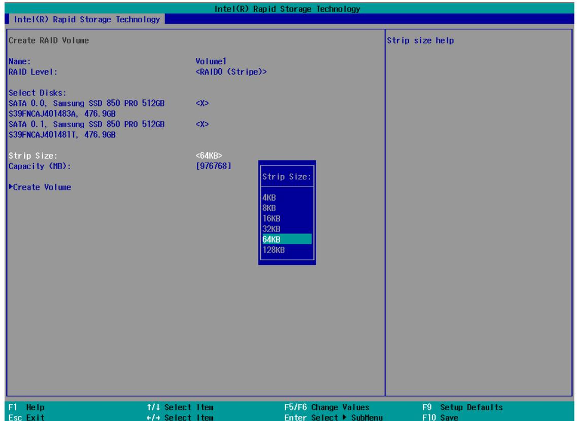
12. The Capacity (MB) option allows you to configure the storage capacity of your RAID volume. By default, the full storage capacity will be applied. Once you have entered a capacity, press ENTER to confirm.
