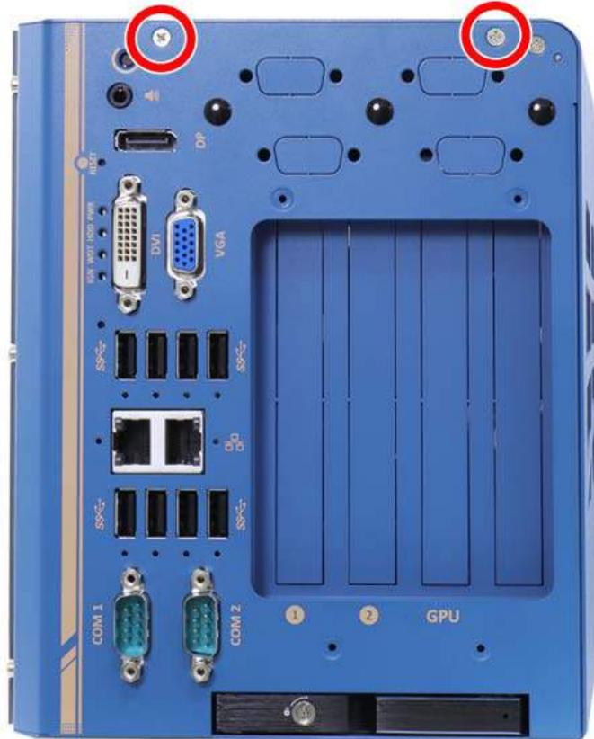
2. Unscrew the screw indicated on top of the enclosure.
