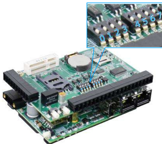
Dip switches on the motherboard. To gain access, please refer to the mini PCIe installation section for system disassembly.
