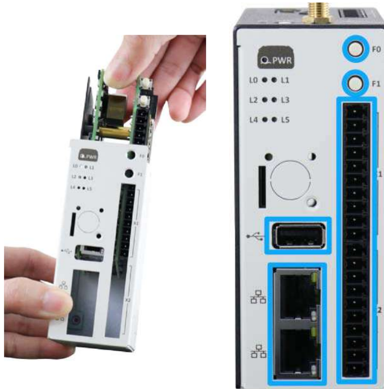
Slide back into enclosure
