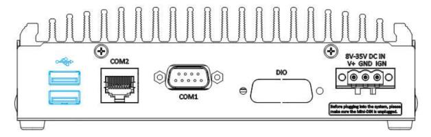
The system has two USB 2.0 ports. They are implemented by native xHCI (eXtensible Host Controller Interface) controller in H310 chipset and are compatible with USB 2.0, USB 1.1 and USB 1.0 devices. Legacy USB support is also provided so you can use USB keyboard/mouse in DOS environment.
