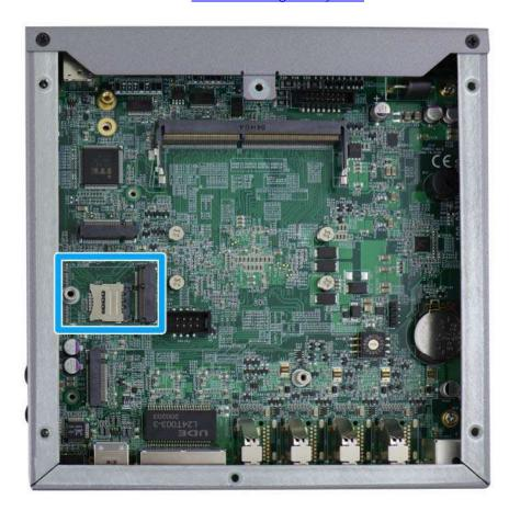
1. To install the M.2 2230 E key module, insert the module on a 45° angle and secure the module using the screw provided.
