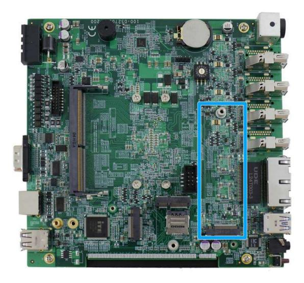
The system has an M.2 2280 slot (SATA signal only) for you to install an M.2 SATA SSD for faster access over traditional hard disk drives.
