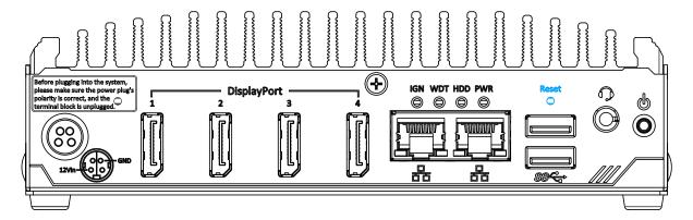
The reset button can be used to manually reset the system in case of abnormal condition. To avoid unexpected operation, the reset button is hidden behind the front panel. You need to use a pin-like object to push the reset button.
