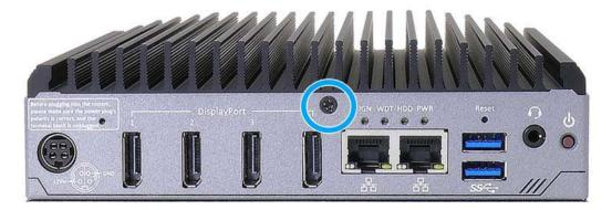
5. Remove the screws from both sides of the chassis.
