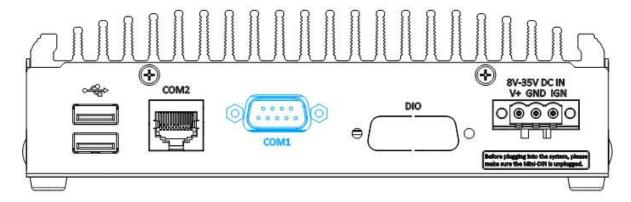
The system provides two COM ports for communicating with external devices. COM1 port is an RS-232 port and you may refer to the following table for its pin definition.
