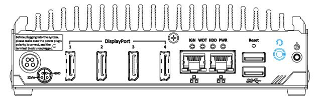
There is a female 4-pole audio jack for headphone (speaker) output and microphone input. To utilize the audio function in Windows, you need to install corresponding drivers. Please refer to the section, <u>Driver Installation</u>.
