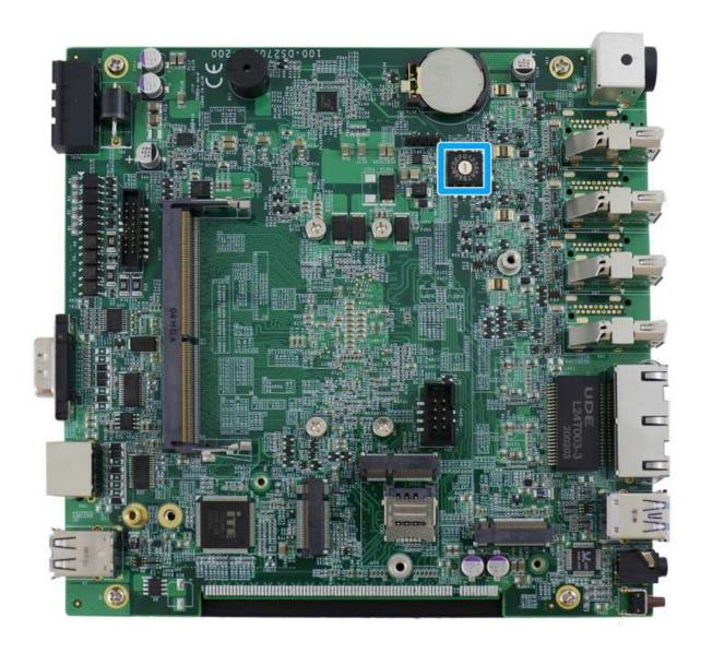
The system features an ignition control switch that has multiple modes for pre and post ignition settings. Please refer to the section <u>Ignition Power Control</u> for details.
