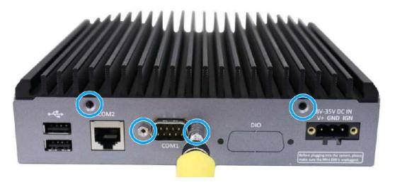
4. Remove the screw indicated on the front I/O panel.
