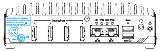
The system accepts a DC power input of 12V. DO NOT plug in the 12V DC connector and the 3-pin terminal connector. The system only requires one or the other for operation.
