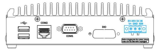
The system accepts a wide range of DC power input from 8 to 35V via a 3-pin pluggable terminal block, which is fit for field usage where DC power is usually provided. The screw clamping mechanism on the terminal block offers connection reliability when wiring DC power.
