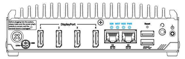
There are four LED indicators on the I/O panel: PWR, WDT, HDD and IGN. The descriptions of these LEDs are listed in the following table.
