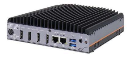
The wide operating temperature and fanless design make it ideal for 24/7 applications in harsh indoor and outdoor environments, such as flight information display system (FIDS) or train schedule board on the platform. Furthermore, Nuvo-2700DS is perfect for stationary or mobile applications due to ignition power control and full bandwidth support of WIFI 6, 4G LTE, and 5G network modules.
