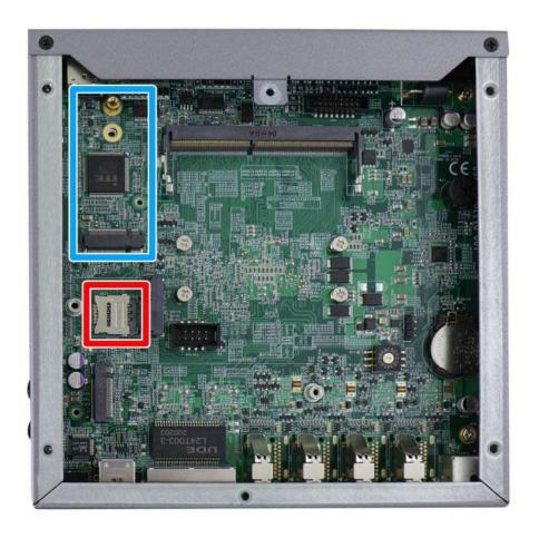
To install the micro-SIM SIM card, slide the metallic cover in the direction shown and lift it to expose the socket and gold fingers.
