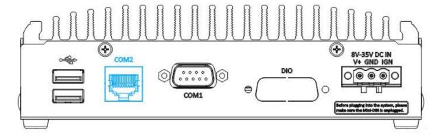
COM 2 port is a RS-232 port that uses an RJ 50 connection. The RJ 50 connection is designed to be compatible with existing digital signage players.
