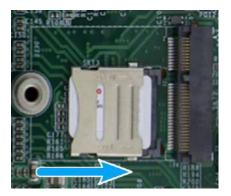
Place into socket with orientation shown Slide cover to secure the micro-SIM
