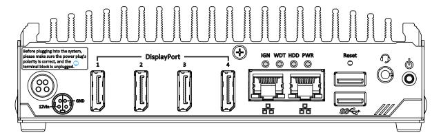
The CMOS Reset button is used to manually reset the motherboard BIOS in case of system halt or malfunction. To avoid unexpected operation, it is purposely placed behind the panel. To reset, please use the tip of a pen, press and hold for at least 5 seconds to reset the BIOS.
