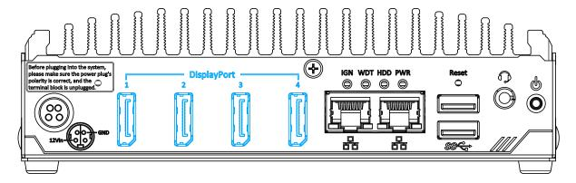
The system has four DisplayPort (DP) outputs which are digital display interfaces that mainly connect video source and carry audio to a display device. When connecting a DP, it can deliver up to 4K UHD (4096 x 2304) in resolution. The system is designed to support passive DP adapter/ cable. You can connect to other display devices using DP-to-HDMI cable or DP-to-DVI cable.
