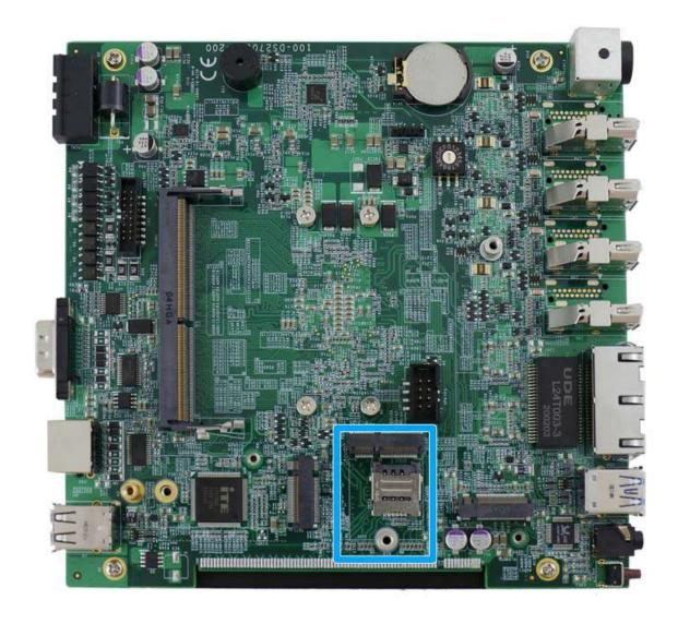
The system has an M.2 2230 E key socket that offers PCIe Gen3 x1 and USB2.0 signal for WiFi module installation.
