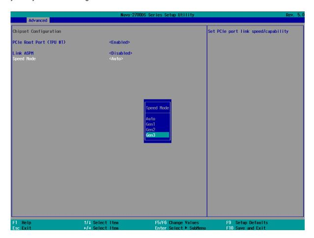
To configure PCIe Root Port (TPU):
