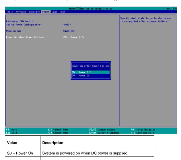
To set "Power On after Power Failure" option:
