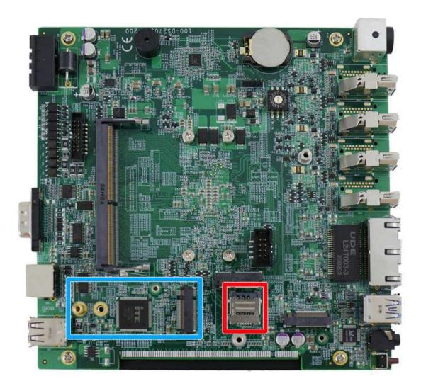
The system has one M.2 3042/ 3052 B key socket (in blue) with USB3.1 Gen 1 and USB 2.0 signal for 4G/ 5G module installation. There is also a corresponding micro-SIM SIM card slot (in red).
