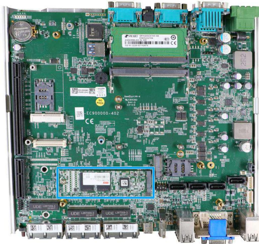
The system has a x4 PCIe M.2 2280 slot for you to install an NVMe SSD for the ultimate performance or an Intel® Optane™ memory to accelerate the read/ write performances of traditional hard disk drive. An NVMe SSD offers exceptional performance over 2.5" SSDs while Intel® Optane™ memory can dramatically boost your traditional hard disk drives' read/ write performances. For installation, please refer to the following instructions.
