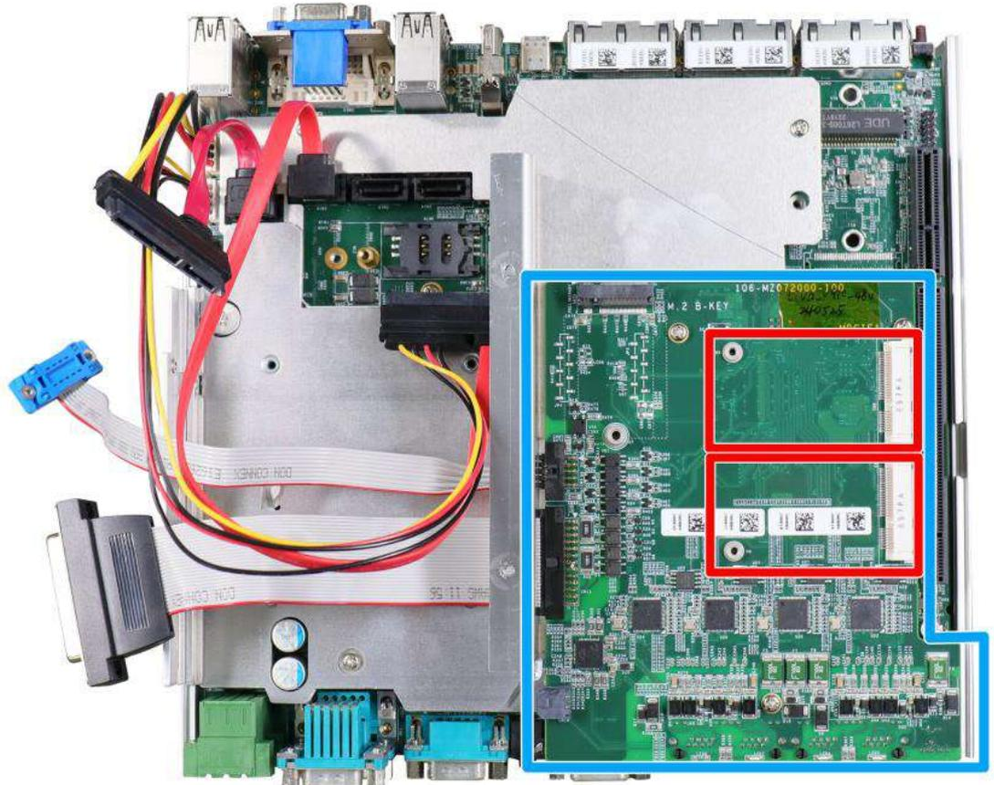
There are two additional full-size mini-PCIe sockets (indicated in **red**) available on the MeziO™ module (indicated in **blue**). They are implemented with USB signals only have better compatibility with off-the-shelf 3G/ 4G mini-PCIe modules. For customers who want to install 3G/ 4G module(s), please take advantage of these two mini-PCIe sockets and the associated SIM slots.
