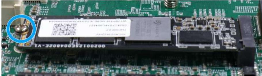
4. Please remember to remove the thermal pad protector film off the heatsink/ support frame for NVMe SSD.
