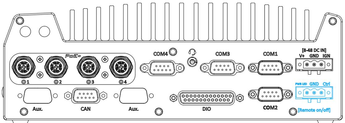
3. With DC power connected, pushing the power button will turn on the system and the PWR LED indicator will light up. Pushing the button when system is on will turn off the system. If your operating system supports ATX power mode (i.e. Microsoft Windows or Linux), pushing the power button while the system is in operation will result in a pre-defined system behavior, such as shutdown or hibernation.
