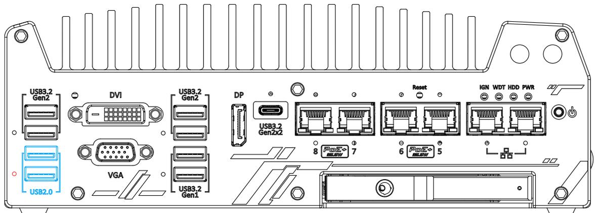
The USB2.0 ports are implemented via native xHCI (eXtensible Host Controller Interface) and are backward compatible with USB 1.1 and USB 1.0 devices. UEFI USB support is also provided so you can use USB keyboard/ mouse in UEFI shell environment. Indicated in **red** is a screw-lock hole for the corresponding USB port.
