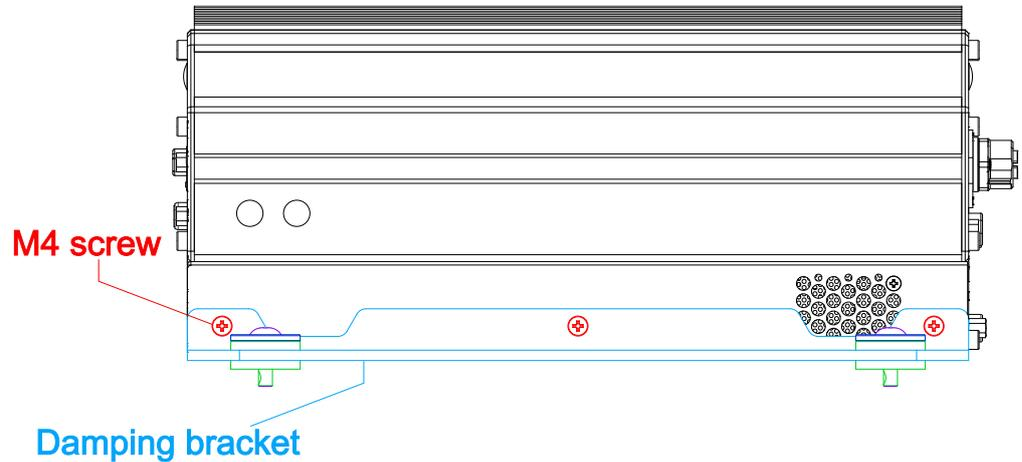
2. Place the system on a flat surface, insert the **sleeves** into the **anti-vibration grommets** and secure it with **M4 screws**.
