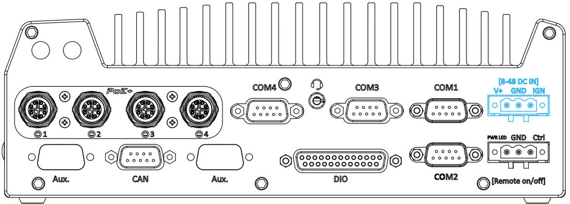
The system accepts a wide range of DC power input from 8 to 48V via a 3-pin pluggable terminal block, which is fit for field usage where DC power is usually provided. The screw clamping mechanism on the terminal block offers connection reliability when wiring DC power.
