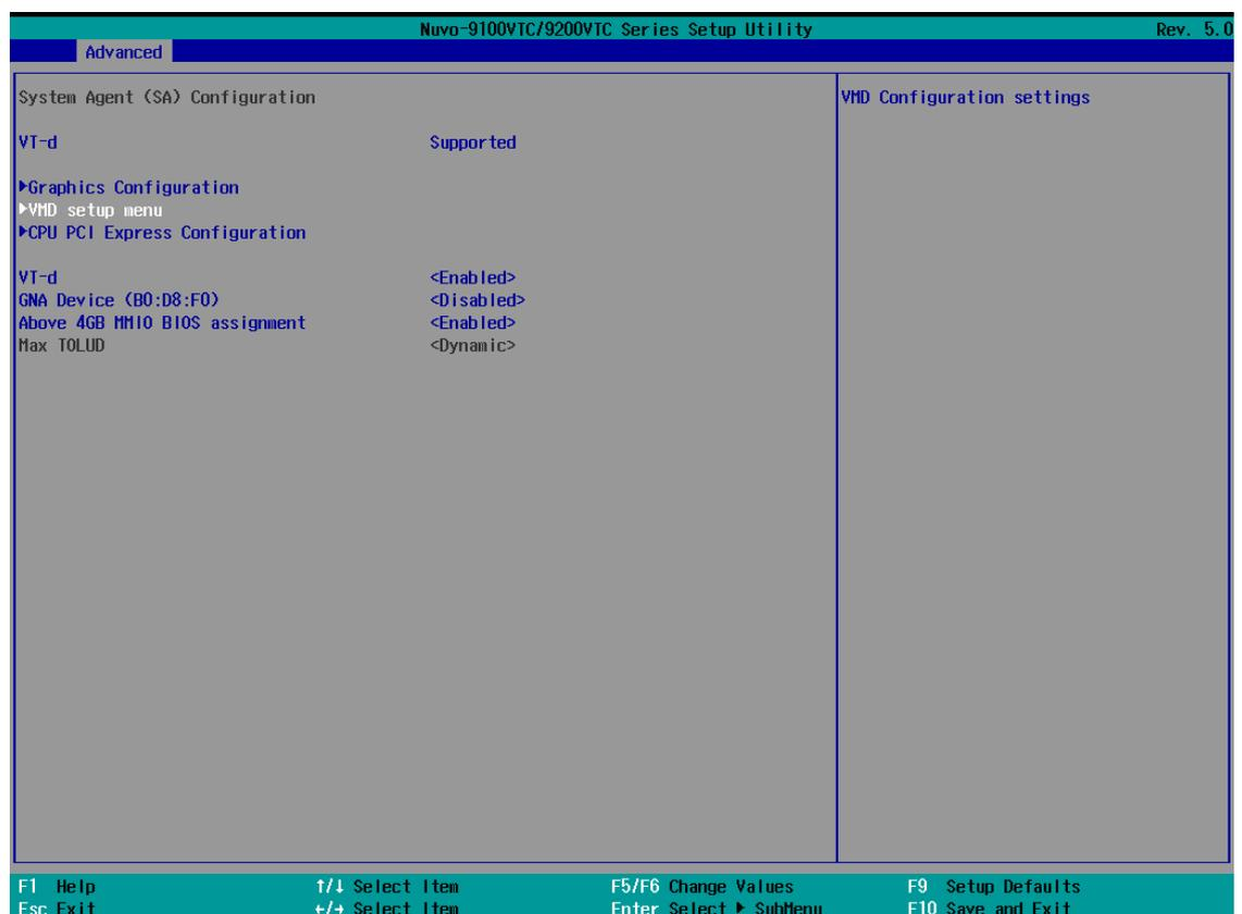
3. Select **[Enable VMD controller]** and press ENTER, highlight **[Enabled]** and press ENTER.
