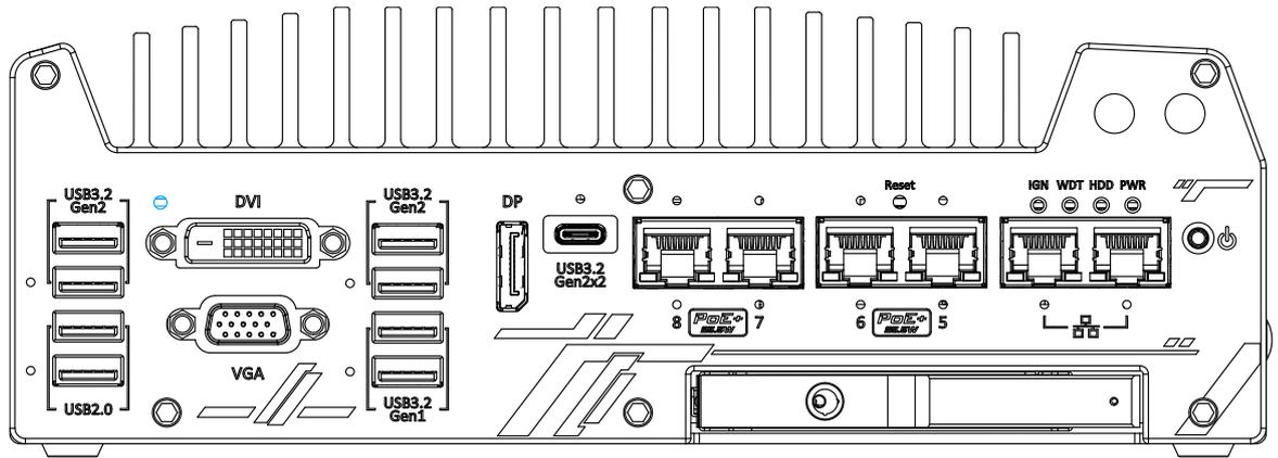
The CMOS Reset button is used to manually reset the motherboard BIOS in case of system halt or malfunction. To avoid unexpected operation, it is purposely placed behind the panel. To reset, disconnect the DC power input, and use the tip of a pen to press and hold for at least 5 seconds to reset the BIOS.
