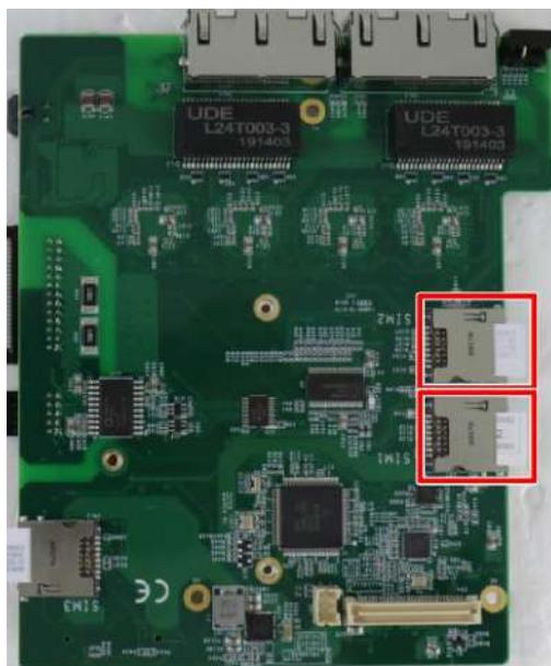
Micro SIM slots are inserted underneath the
