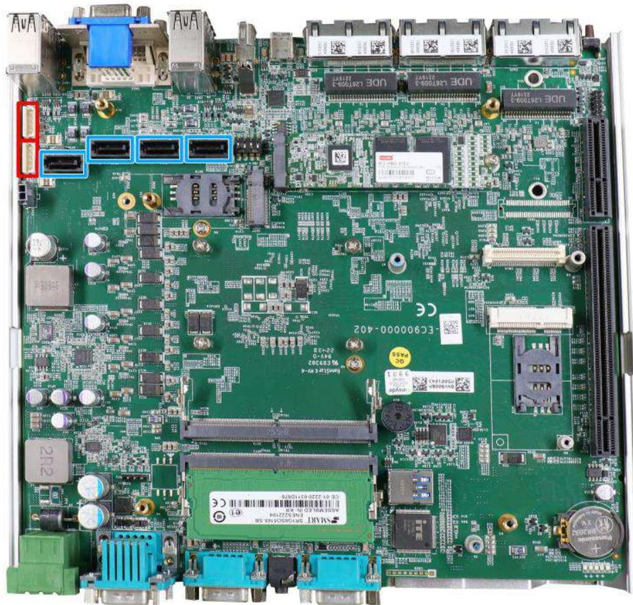
The system has SATA ports (blue) and four-pin power connectors (red). The SATA and power cables should already be connected on the motherboard so users only need to install the 2.5" SATA HDDs/ SSDs to the front hot-swappable tray(s). For Nuvo-9100VTC systems, there is also an internal drive that can be coupled to configured into RAID 0 or 1 storage. If you previously disconnected the SATA and power cables, please reconnect them before continuing with this installation procedure.
