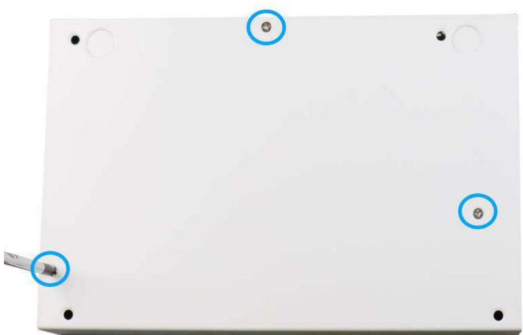
7. Gently lower the Cassette module back onto the system enclosure and secure the module onto the system enclosure by securing the following screws.
