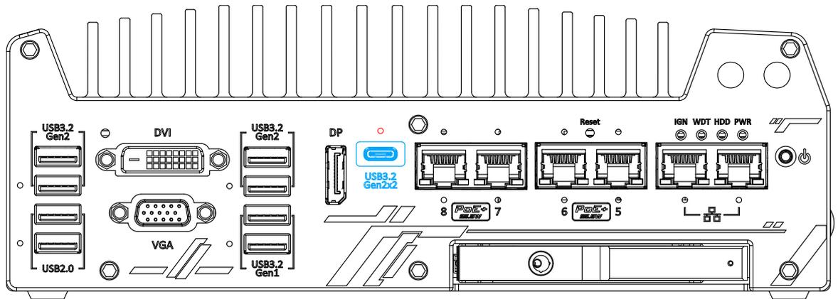
The system's USB 3.2 Gen2x2 type-C port offers up to 20Gbps of data transfer bandwidth, and is implemented via the native xHCI (eXtensible Host Controller Interface) controller. Indicated in **red** is a screw-lock hole for the corresponding USB port.
