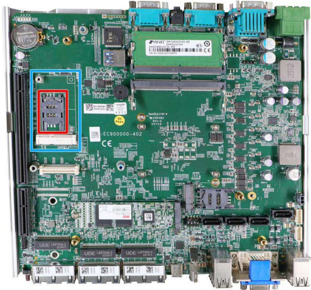
The system provides a mini-PCle socket (indicated in blue) that is in compliance with mini-PCle specification rev. 1.2. This mini-PCle socket is designed with SIM card (slot indicated in red) support. With a SIM card installed, your system can access the internet via your network provider's 4G/ 3G network.
