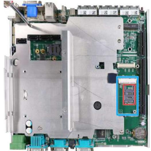
mini-PCIe slot on motherboard
