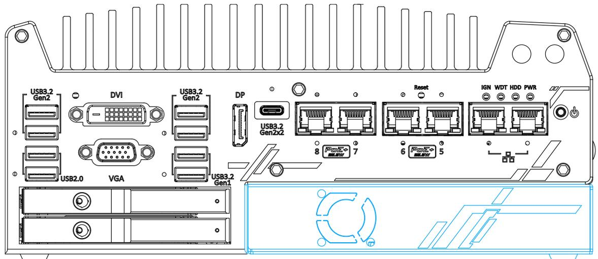
Neosys' patented expansion Cassette (R.O.C. Patent No. M456527) provides a separated compartment to accommodate an add-on card. It effectively manages thermal conditions of both the system and the add-on card. The modular concept brought by Cassette module also reduces the complexity of installing and replacing an add-on card in the fanless controller.
