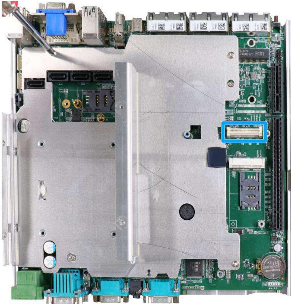
MezIO™ is an innovative interface designed for integrating application-oriented I/O functions into an embedded system. It offers computer signals, power rails and control signals via a high-speed connector. MezIO™ is also mechanically reliable benefited from its 3-point mounted mezzanine structure. A MezIO™ module can leverage these signals to implement comprehensive I/O functions.
