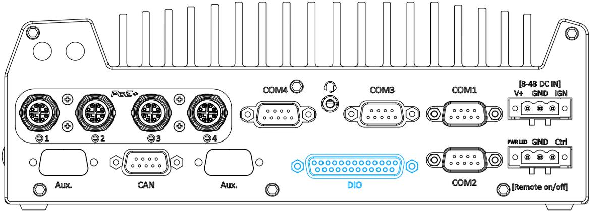
The system provides 4x isolated digital input channels and 4x isolated digital output channels. The DIO functions support polling mode I/O access and DI change-of-state interrupt. Please refer to digital I/O pin definition on the following page and [Watchdog Timer & Isolated DIO](#) for information on wiring and programming the isolated DIO channels.
