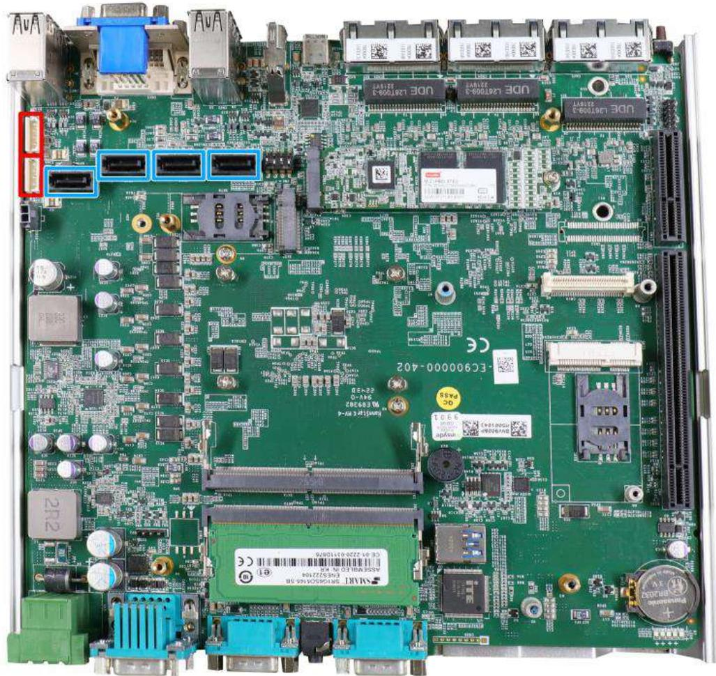
The system has SATA ports (indicated in blue) and four-pin power connectors (indicated in red). The SATA and power cables should already be connected on the motherboard so users only need to install the HDD/ SSD. Please refer to the following instructions on how to install 2.5" SATA HDD/ SSD.
