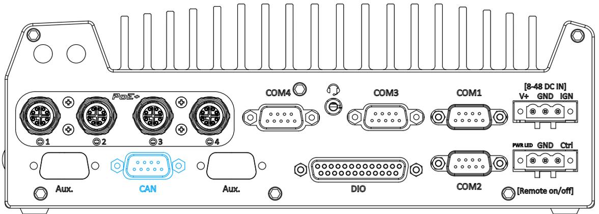
CAN bus is a robust industrial bus with a pair of differential signals and is commonly used in various industrial and in-vehicles applications. The system is equipped with a CAN bus DB9 port that is compatible with both industrial and in-vehicle applications. The CAN bus port supports CAN2.0A and CAN2.0B up to 1Mbps.
