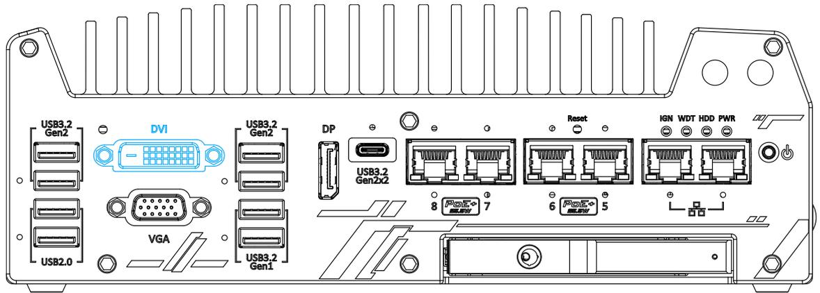
DVI-D transmits graphics data in digital format and therefore can deliver better image quality at high resolution. The DVI connector on the front panel can either output DVI signals or other digital signals (via an adapter/ cable) depending on the display device connected. It supports resolutions up to 1920x1200@60Hz.
