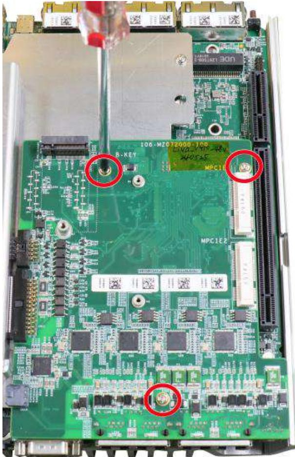
10. Once the MezIO™ module has been separated, remove the heatsink/ support frame by removing the screws shown below.
