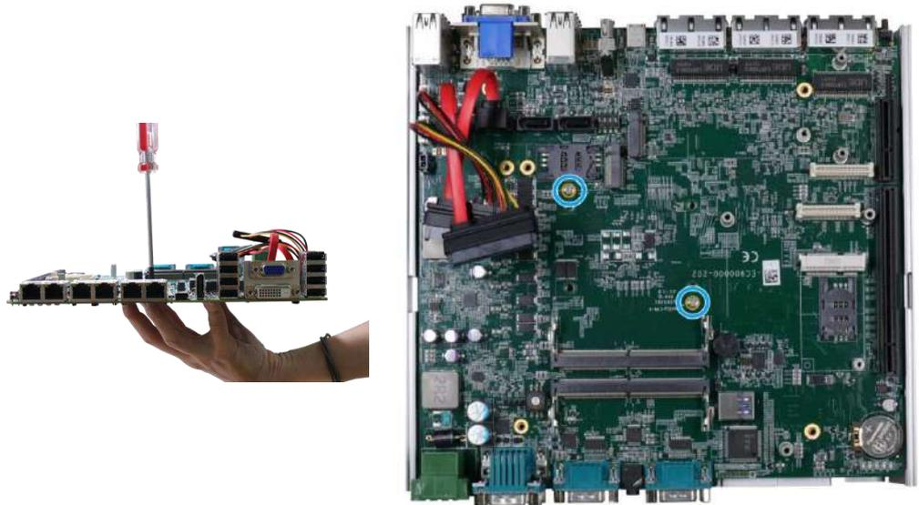
**Hold CPU bracket firmly and turn the motherboard around**
