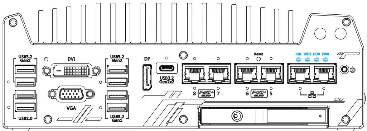
There are four LED indicators on the I/O panel: IGN, WDT, HDD and PWR. The descriptions of these four LED are listed in the following table.
