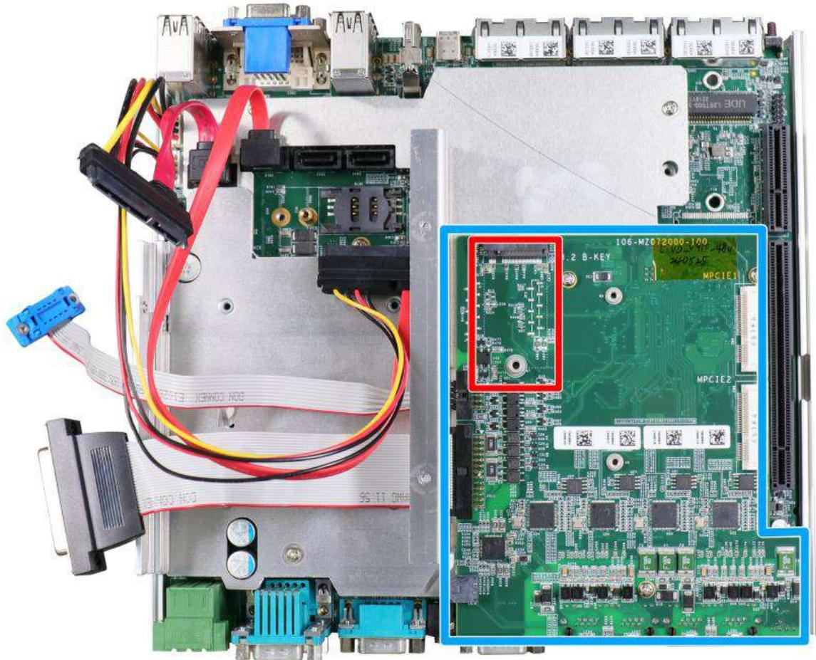
There is an additional M.2 2242 slot (indicated in red) available on the MeziO™ module (indicated in blue). To expand wireless networking capability, users can install off-the-shelf 4G/ 3G modules and access the internet via the provider’s network.
