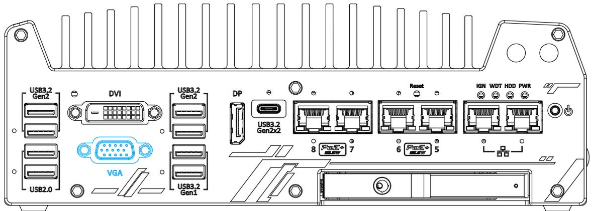
VGA connector is the most common video display connection. The VGA output supports up to 1920x1200@60Hz resolution.
