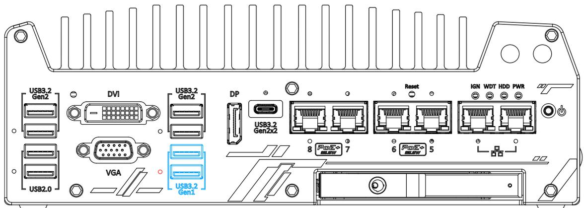
The system's USB 3.2 Gen1x1 ports (5Gbps) are implemented via native xHCI (eXtensible Host Controller Interface) controller and are backward compatible with USB 2.0, USB 1.1 and USB 1.0 devices. UEFI USB is also supported so you can use USB keyboard/mouse in UEFI shell environment. Indicated in **red** is a screw-lock hole for the corresponding USB port. xHCI driver is supported natively in Windows 10, therefore you do not need to install the xHCI driver prior to utilizing USB functions.
