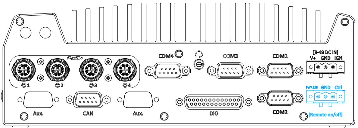
The “Remote On/ Off” 3-pin connection allows for external switch extension. It is useful when the system is placed in a cabinet or a not easily accessed location. You may connect an external status LED (20mA) indicator by connecting to PWR LED and GND.
