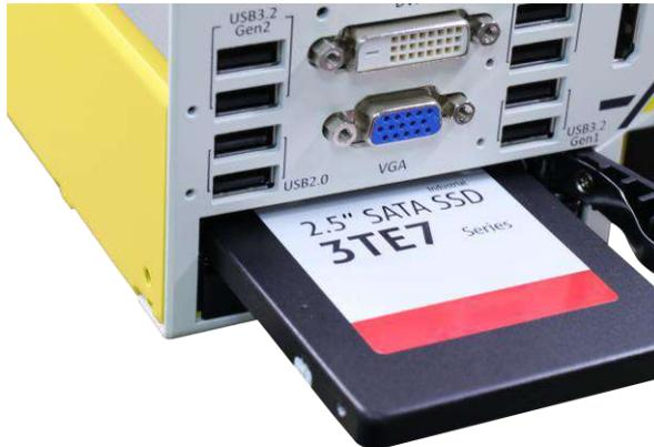
3. Push the lever into the 2.5" slot until it snaps into position. A key is provided (in accessory box) to lock the external slot.
