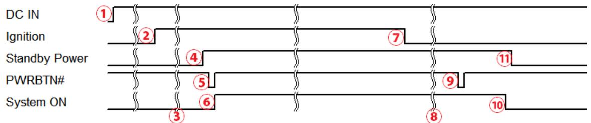
1. When DC power is supplied to the system, MCU starts to periodically detect ignition signal.
