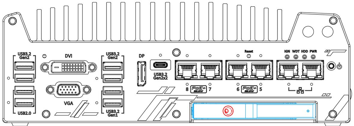
The Nuvo-9100VTC systems support an external 2.5” HDD/ SSD via a hot-swappable slot. Designed for easy access, the HDD/ SSD slot is secured by a lock (indicated in red) and it supports RAID modes 0/ 1 configuration by combining with the internal HDD/ SSD drive for OS installation (coupled with the internal HDD). To set up RAID, please refer to RAID Volume Configuration section for details.
