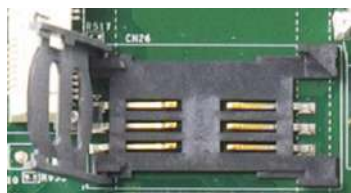
Slide and lift SIM card holder
