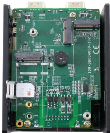
Place micro SIM in slot
