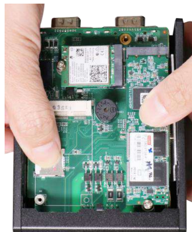
Secure micro SIM with cover
