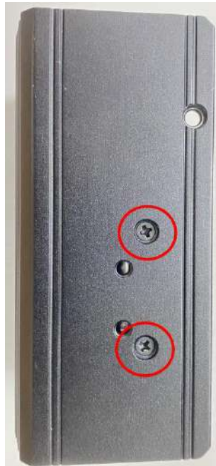
Remove the screws
