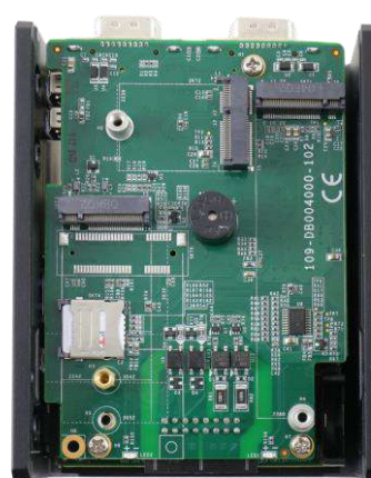
Secure micro SIM with cover
