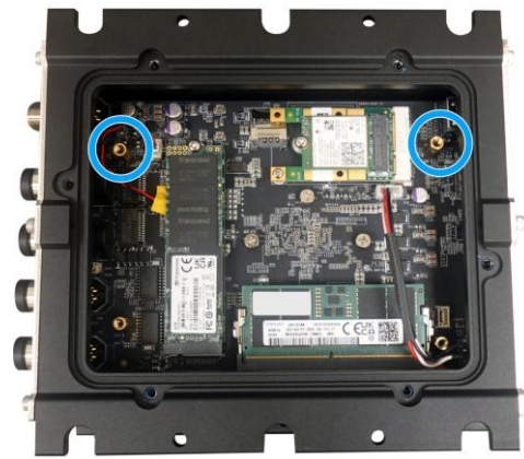
Install the copper stand-offs
